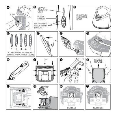
To start clipper, move power switch to ON position. To stop clipper, move power switch back to original position (Figure B).
